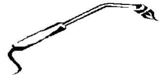
Before lighting the torch, test the system for leaks with soapy water. Using a spray bottle to apply the soapy water. Remember, you need to be wearing proper gloves and goggles and ensure that the area in which you are using the torch is safe.
